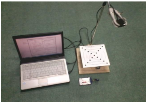
Gambar 8. Sistem pengendalian ball on plate balancing system lengkap
