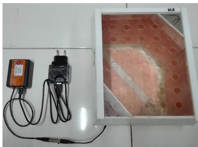
Figure 1. ECCT device for animal study. The size of the cage is 23 \text{ cm} \times 18 \text{ cm} \times 19 \text{ cm} . The electrodes are attached to the acrylic wall of the cage with opposite polarity facing each other to produce multiple field directions.
