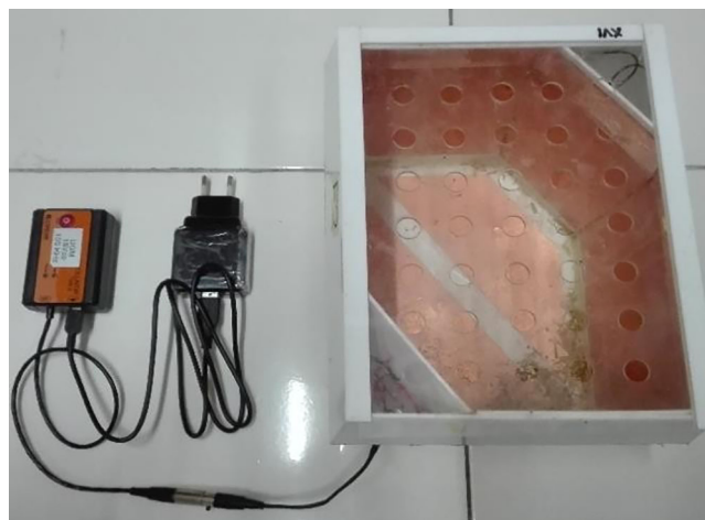
Figure 1. ECCT device for animal study. The size of the cage is 23 cm × 18 cm × 19 cm. The electrodes are attached to the acrylic wall of the cage with opposite polarity facing each other to produce multiple field directions.
