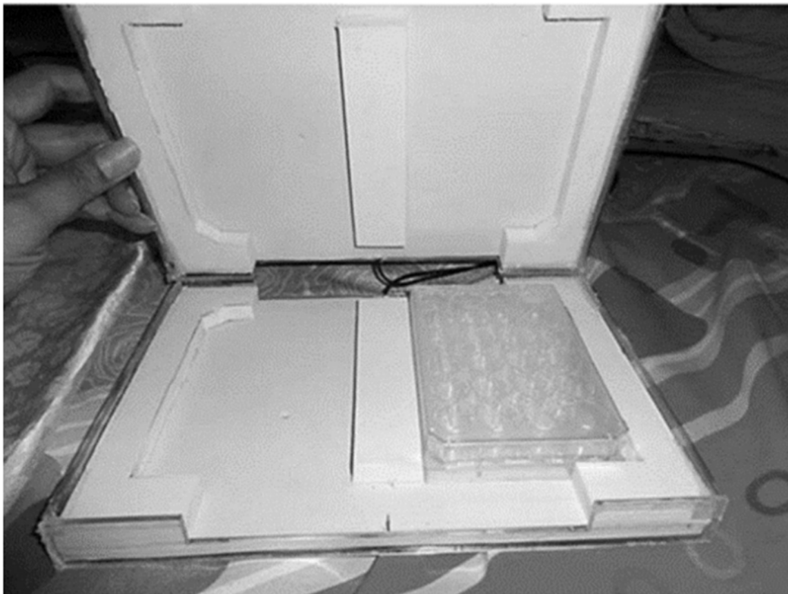
Figure 1. Capacitive electrodes as electrical field generator. A microplate was flanked between two capacitive electrodes that were connected to low intensity oscillator to generate the alternate electric field
