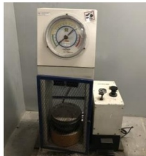
Figure 6. Compression testing machine
