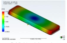
Fig. 2. Simulation result of warpage at base
