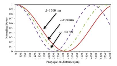
Figure 5 Power transfer as a function of propagation distance with different wavelengths.
