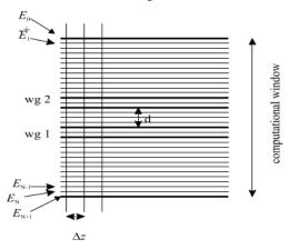
Figure 1 MoL discretization scheme used for the example of a directional coupler.
