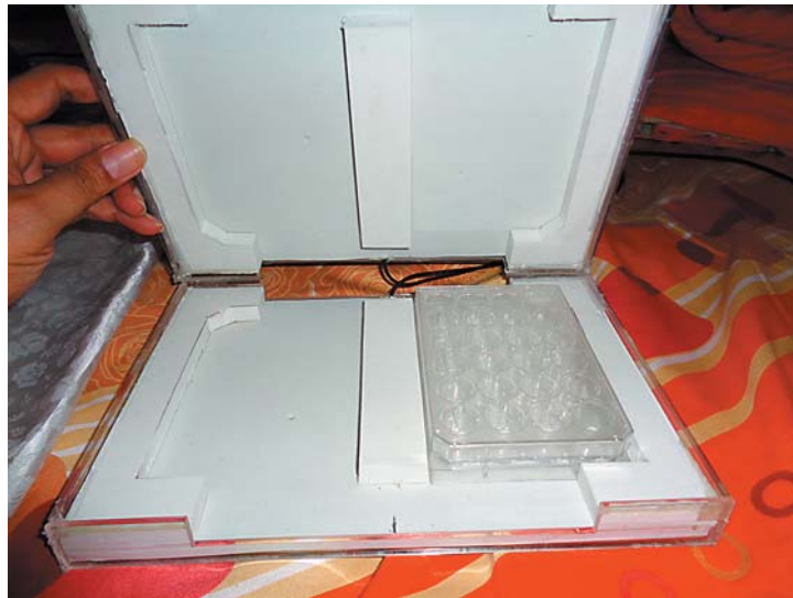
Fig. 2. A microplate flanked by 2 capacitive electrodes.
